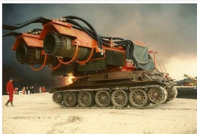
Image from Romanian video of 1991 Kuwaiti oilfields: “Twin MIG-21 turbojets mounted on a World War II era Soviet T-34 tank dubbed “Big Wind” generated 700 mph thrust blasting hundreds of gallons of water per second into the fire.”
