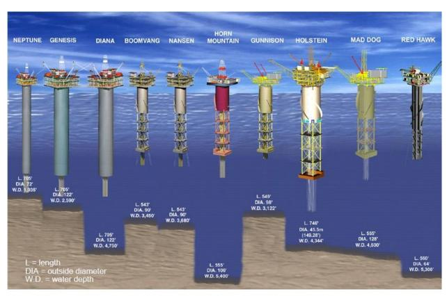
Figure 43. Progression of spar deepwater development systems (image courtesy of Technip-Coflexip).
