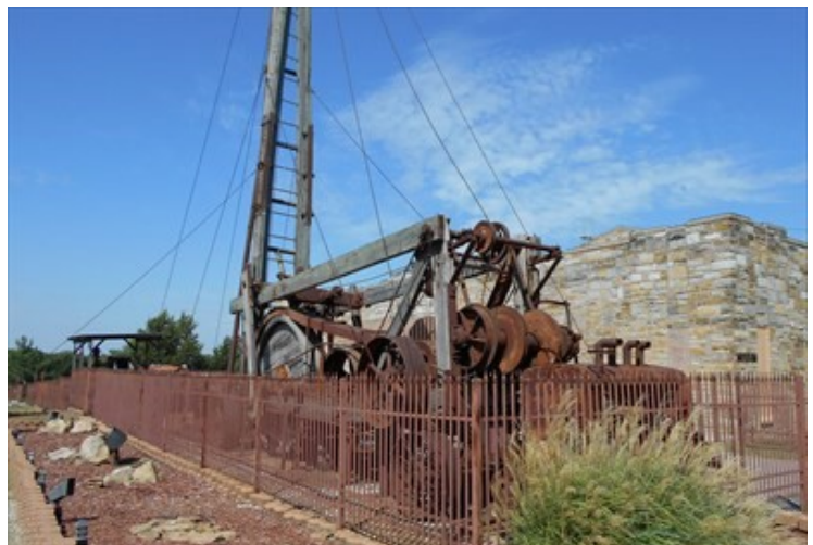
Spudder Drilling Rig—Manufactured in Wichita Falls
