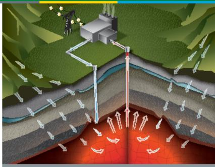
Geothermal energy, accessed through fluid in the hot rocks at a depth up to several miles, supplies a steady flow of high-pressure steam or water to create electricity.
